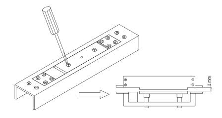
After mounting, adjust the adjusting screws to make sure the gap is 3mm as drawing above.
